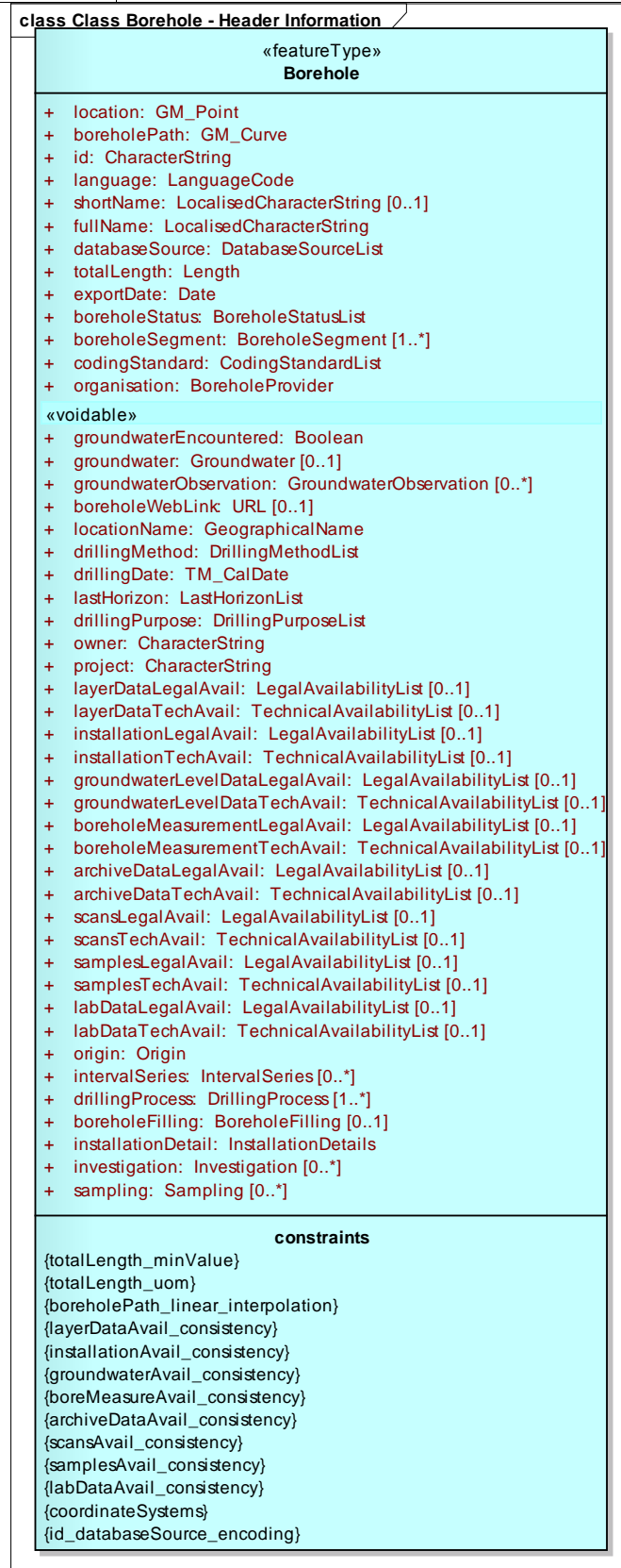
Figure 6: Class Borehole - Header Information
